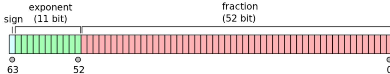
The real value assumed by a given 64-bit double-precision datum with a given **biased exponent**  $e$  and a 52-bit fraction is
